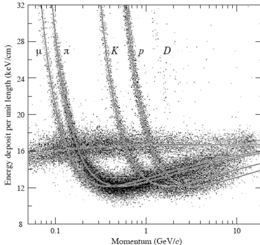
**Figure 28.8:** PEP4/9-TPC energy-deposit measurements (185 samples @8.5 atm Ar-CH<sub>4</sub> 80–20%) in multihadron events. The electrons reach a Fermi plateau value of 1.4 times the most probably energy deposit at minimum ionization. Muons from pion decays are separated from pions at low momentum;  $\pi/K$  are separated over all momenta except in the cross-over region. (Low-momentum protons and deuterons originate from hadron-nucleus collisions in inner materials such as the beam pipe.)
