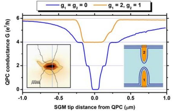
**Fig.1** Conductance profile through the QPC as a function of filling factors  $g$  under the QPC gates. The left inset shows a two-dimensional SGM map of  $G$  vs. tip position for  $g_1 = g_2 = 0$ . The vertical line indicates the profile position, the QPC border is outlined. The right inset is a sketch of the edge channels for  $g_1 = 2, g_2 = 1$ .
