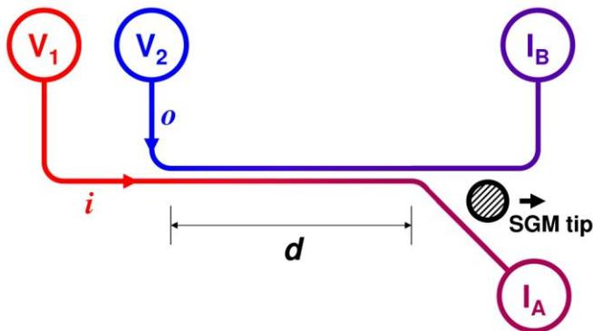
Figure 1 schematically illustrates our experiment: inner ( $i$ ) and outer ( $o$ ) edge channels originate from two distinct voltage contacts at potential  $V_1$  and  $V_2$ , respectively. They propagate together for a distance  $d$  and are then separated and guided to two current contacts  $I_A$  and  $I_B$ , respectively. In what follows we set  $V_1 = V$  and  $V_2 = 0$ . If we assume that there is no equilibration between the two (spin-degenerate) edge channels, then  $I_A$
