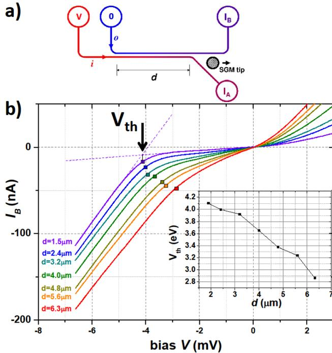
Fig. 1: (a) Sketch of the experimental setup. (b) I-V characteristics of the inter-channel equilibration. In the inset the threshold energy reduction as a function of  $d$  is shown.
